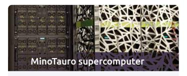
Heterogeneous cluster with NVIDIA GPUs. 343.74 Teraflops top speed.
